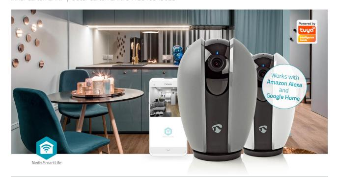
This easy to use Smart Indoor IP Camera with a pan and tilt functionality to cover the whole room can be simply connected to your existing Wi-Fi network to monitor rooms of your house and record any sound or motion, whether you are at home or on the road. The Nedis SmartLife app notifies you in case of movement and noise, so you can intervene in time.
