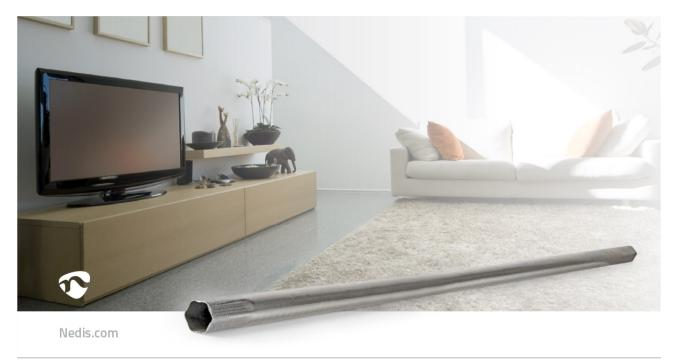
Satellite mast made of galvanised steel to mount aerials or dishes. The mast has a diameter of 42 mm and a length of 2 m. A telescopic system enables easy extension by attaching two Nedis masts to each other.
